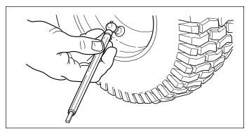
Figure 10. Checking Tire Pressure
